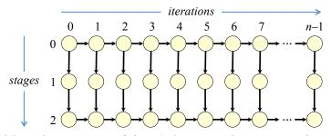
**Figure 7-1:** Modeling the execution of *ferret*'s linear pipeline as a pipeline dag. Each column contains nodes for a single iteration, and each row corresponds to a stage of the pipeline. Vertices in the dag correspond to nodes of the linear pipeline, and edges denote dependencies between the nodes. Throttling edges are not shown.
