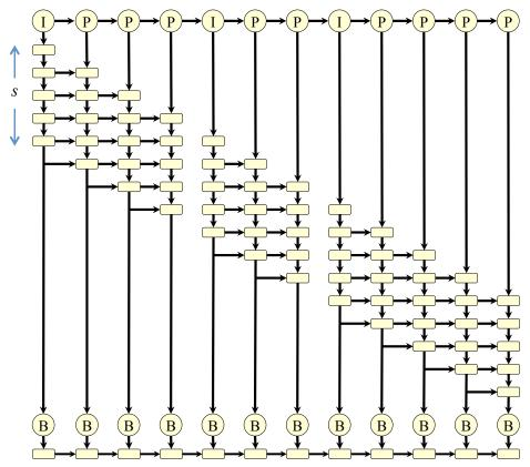
Figure 7-3: The pipeline dag generated for x264. Each iteration processes either an I- or P-frame, each consisting of s rows. As the iteration index i increases, the number of initial stages skipped in the iteration also increases. This stage skipping produces cross edges into an iteration i from null nodes in iteration i - 1. Null nodes are represented as the intersection between two edges.
