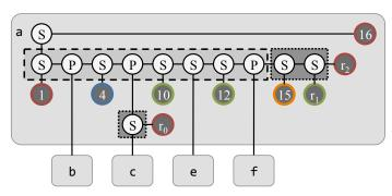
**Figure 9-9:** The spawn parse tree for the performance dag in Figure 9-5. This spawn parse tree augments the SP parse tree in Figure 9-4 with reduce chains, which are indicated by the dark rectangles outlined by dotted lines. Strands, which appear at the leaves of the tree, are labeled with either their label in Figure 9-2 or, for reduce strands, by their label  $r_0$ ,  $r_1$ , or  $r_2$  in Figure 9-5. Strands with the same view ID are colored similarly, as in Figure 9-5.
