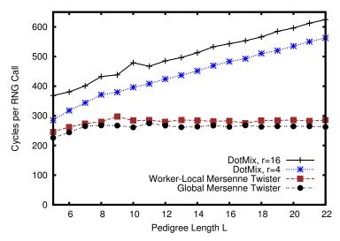
**Figure 6-8:** Overhead of various RNG's on the CBT benchmark when generating  $n = 2^{20}$  random numbers. Each data point represents the minimum of 20 runs. The global Mersenne twister RNG from the GSL library [147] only works for serial code, while the worker-local Mersenne twister is a nondeterministic parallel implementation.
