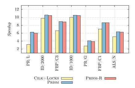
Figure 4-10: Empirical speedup relative to SERIAL-DDGC on 12 processor cores. Shown are the empirical speedups  $T_s/T_{12}$  of CILK+LOCKS, PRISM, and PRISM-R, where  $T_s$  is the running time of the serial scheduling algorithm SERIAL-DDGC and  $T_{12}$  is the running time of the particular algorithm on 12 cores. The PRISM-R algorithm is discussed in Section 4.6.
