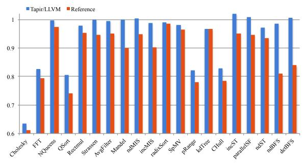
Figure 10-16: The work efficiency of Tapir/LLVM and the Reference compiler. For each compiler, the bar for each benchmark shows the ratio  $T_S/T_1$ , where  $T_s$  is the running time of the serial elision of the benchmark, and  $T_1$  is the running time of the parallel Cilk code on 1 processor core.
