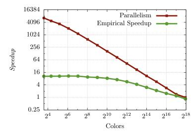
Figure 4-11: Scalability of PRISM on the image-denoise application as a function of  $\chi$ , the number of colors used to color the data graph. The parallelism  $T_1/T_{\infty}$  is plotted together with the empirical speedup  $T_1/T_{12}$  achieved on a 12-core execution. Parallelism values were measured using the Cilkview scalability analyzer [180].
