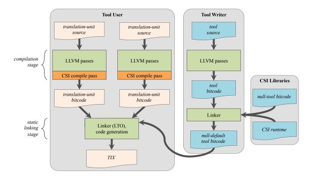
**Figure 11-11:** The implementation of CSI:LLVM. Gray rounded rectangles distinguish the concerns of the tool user, the tool writer, and the CSI-provided libraries. The tan shapes represent code (in some form) for the program-under-test. The blue shapes represent code for the tool or the CSI system itself. The green boxes are compiler, linker, and code-generation components already provided by LLVM. The orange boxes indicate new LLVM passes that implement CSI.
