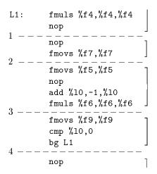
**Figure 3-14**: Assembly code loop produced by exchanging two instruction in the code in Figure 3-13, which cannot execute at the rate of 4 instructions per cycle because of the grouping limitation.
