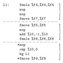
**Figure 3-13**: Assembly code loop which is executed at the maximum execution rate of 4 instructions per cycle.
