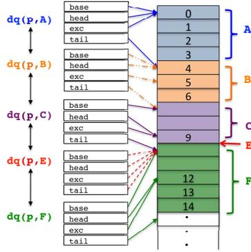
**Figure 5.** A chain of dequeues for a given worker  $p$ . Each deque  $dq(p, A)$  consists of pointers (tail, head, and exception) into  $p$ 's stack of Cilk frames. For clarity, we show a pointer for the base of each deque  $q$ , although in practice,  $q$ 's base always equals the tail pointer of  $q$ 's parent deque.
