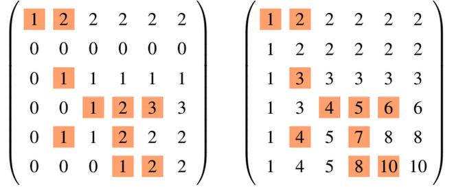
(b) Next, `COMPUTE` $\mathcal{X}$  performs a prefix sum on the rows and then columns of the matrix. Notice that element  $\mathbf{j}$  of the matrix is now equal to the number of nonzero elements in the box extending from the upper left of the matrix to element  $\mathbf{j}$ .
