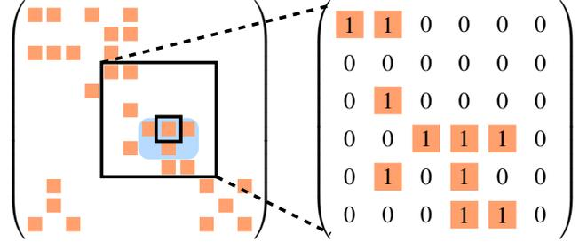
(a) First, `COMPUTE` $\mathcal{X}$  uses `NONZEROSINRANGE` to find the nonzeros within a box of size  $2B$  around  $\mathbf{i}$ . Then, it creates a matrix of the same size as the box and fills it with 0 where there are zeros in the original matrix and 1 where there are nonzeros.
